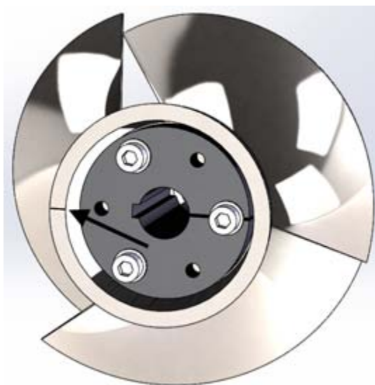
Figure 47. Position of the keyway
