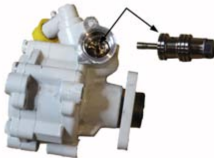
Figure 80. The hydraulic pump and the pressure relief valve
