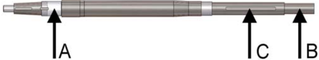
Figure 13. Measuring the straightness of the shaft
