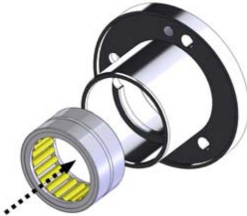
Figure 34. Assembly of the rear bearing
