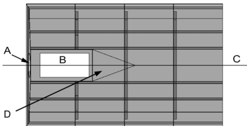
Figure 6. Hole position in relation to keel line
